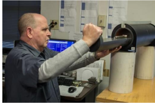
QC Forge performs special magnetic testing on critical relay components to confirm low "magnetic remanence" properties.
