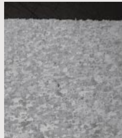
00-1582-03 QC Force 40Min. T-6 Heat Treatment 50X 100µm 100H 2 O / 2g Na 2 MoO 4 ·2H 2 O / 2g NH 4 HF 2 / SHCL
