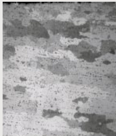
00-1584-01 Finished T-6 Heat Treatment 50X 100µm 100H 2 O / 2g Na 2 MoO 4 ·2H 2 O / 2g NH 4 HF 2 / SHCL
