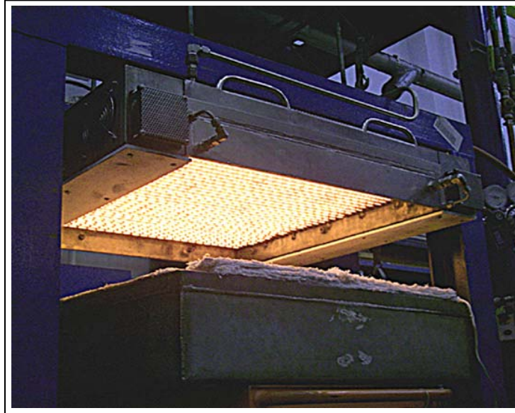
Figure 1. Batch type drop bottom infrared furnace
